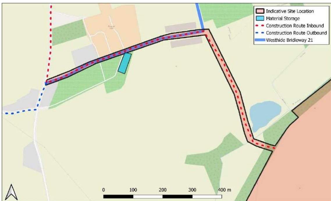
Figure 3.1: Main Construction Access and Layout
